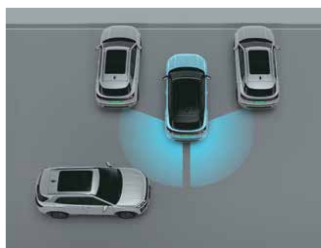
Rear Cross - Traffic Collision - Avoidance Assist (RCCA) & Rear Cross - Traffic Collision Warning (RCCW)
